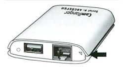
White Remove back cover (side with serial number) by grasping the side edge where indicated and pulling back.
